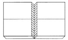
FCAW fill and cap - vertical position using 0.035 flux-cored wire
